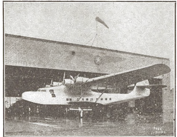
The new Martin Clipper, built by Glenn L. Martin in Baltimore for the Pan-American Airways, is so big it has to be drawn out of the hangar sideways on a special wheeled cradle towed by a tractor. It has recently passed its flight tests and astounded the pilots by the remarkable speed in which it lifts itself clear of the water.
